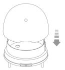
Please make sure the gap of cover is aligned with switches!
